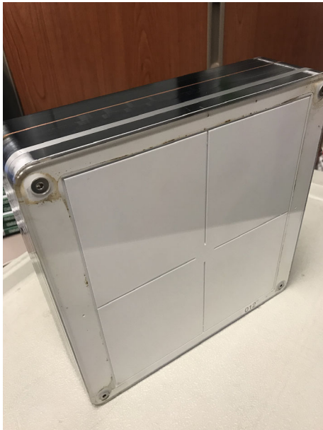
FIG. 3. Custom made, patient equivalent QC phantom or “CD Phantom”.
