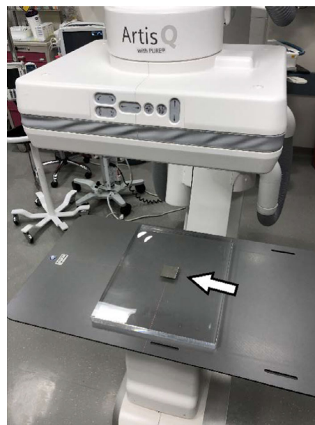
FIG. 1. Tin swatch used for contrast to noise ratio measurement directly on top of 1st sheet of polymethyl methacrylate.
