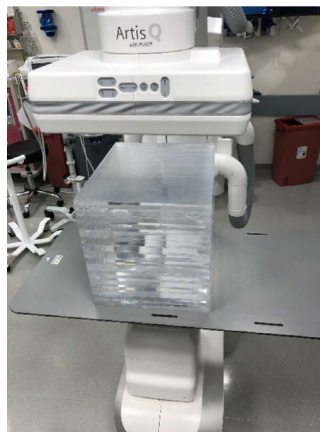
FIG. 2. Slab phantom consisting of a stack of 2.54 cm thick 35.5 cm × 43.2 cm polymethyl methacrylate sheets.
