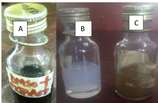
Fig. 1. Visual Observation of SNPs formation: (a) Oscillatoria sp. extract; (b) Silver nitrate solution and (c) SNPs.
