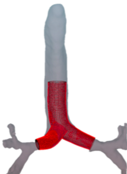
Figure 7 Illustration of the prescription software using a virtual image to build a 3D stent platform. The virtual file generated by a computer-aided design from DICOM that converted to a STL. DICOM, digital imaging and communications in medicine; STL, standard tessellation language.
