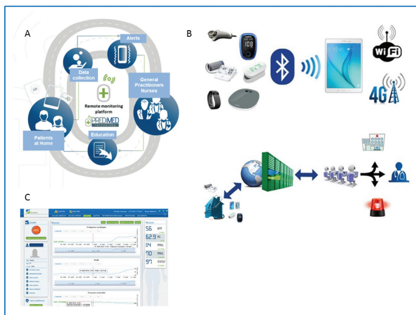
Figure 5: Telemedicine project: DIABETe. A: DIABETe is based on a smart system comprising an inference engine and a medical ontology for personalized synchronous or asynchronous analysis of data specific to each patient and, if necessary, the sending of an artificial intelligence-generated alert (MyPredi™). B: The platform comprises connected non-intrusive medical sensors, a touchscreen tablet connected by Wi-Fi, and a router or 3G/4G, rendering it possible to interact with the patient and provide education on treatment, diet, and lifestyle. C: The system involves a server that hosts the patient’s data and a secure internet portal to which the patient can be connected to hospital- and non-hospital-based healthcare professionals.
