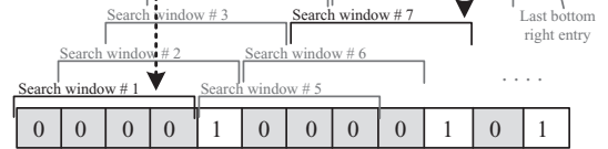
Fig. 1. Neighborhood map ( M ) and the Shouji bit-vector, for text T=GGTGCAGAGCTC and pattern P=GGTGAGAGTTGT for E = 3 . The three common subsequences (i.e. GGTG, AGAG and T) are highlighted in gray. We use a search window of size four columns (two examples of which are highlighted in black) with a step size of a single column. Shouji searches diagonally within each search window for the 4-bit vector that has the largest number of zeros. Once found, Shouji examines if the found 4-bit vector maximizes the number of zeros at the corresponding location of the 4-bit vector in the Shouji bit-vector. If so, then Shouji stores this 4-bit vector in the Shouji bit-vector at its corresponding location
