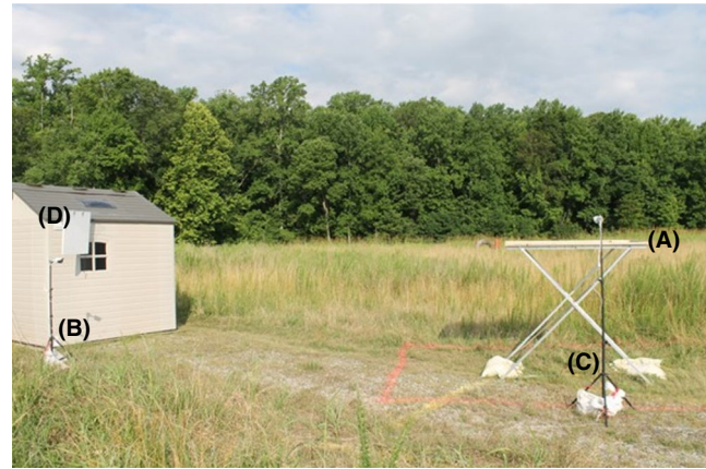
FIGURE 2 This image shows the data capture setup for this field experiment on one side of the experimental area. This setup is mirrored on the other side of the shed. Two CCTV cameras are pointed at the food table (A), one close to the shed to record the entire food table and surrounding area (B) and the other to record the top of the food table (C). The white panel mounted on the shed (D) is the parametric array speaker that allows the sound beam to cover one food table while being inaudible on the other food table
