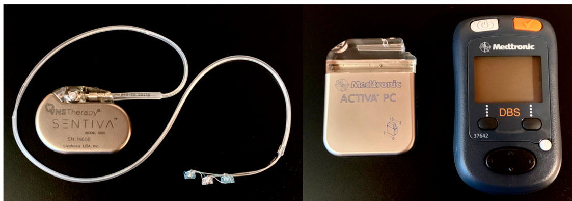
Figure 1. Examples of vagus nerve stimulation (VNS) and deep brain stimulation (DBS) devices. VNS internal pulse generator or neurostimulator (left side of left panel) with extension and coil electrodes (right side of left panel). DBS neurostimulator (left side of right panel) and patient programmer (right side of right panel).
