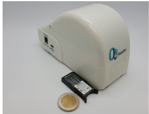
Fig. 1 Q3 platform: the Q3 disposable lab-on-chip cartridge is the core of the system, and is where the Real-Time PCR reactions occur. The Q3 Reader instrument is on the right. Both components are very compact, as shown by comparison with the coin. Dedicated software run on a PC completes the platform
