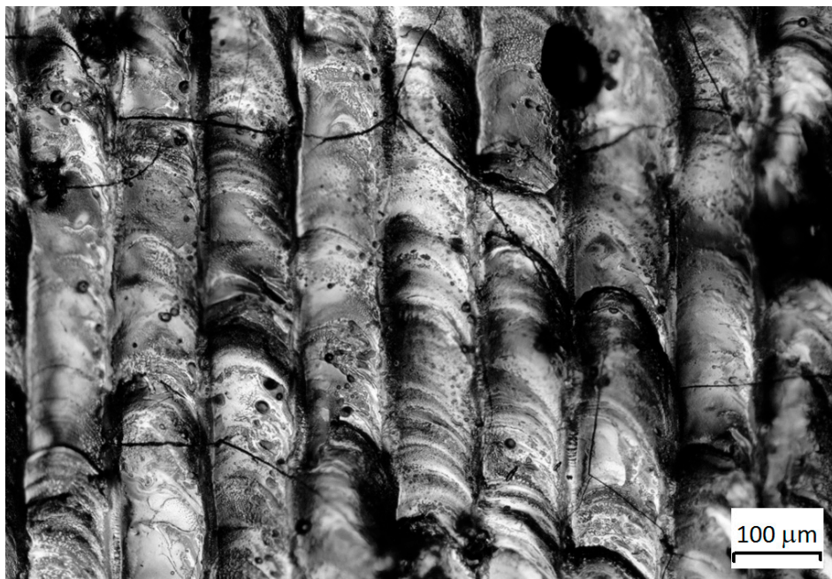
Figure 8. Cracks on the surface of the monolayer—94 wt% WC and 6 wt% Co P = 120 W, V = 300 mm/s.
