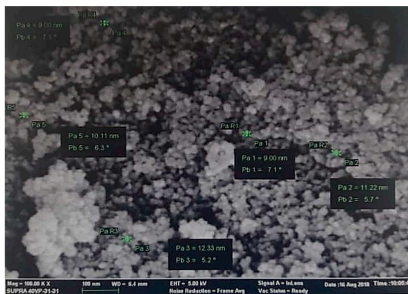
Figure 5. Field emission scanning electron microscopy (FESEM) micrograph of the biosynthesized iron oxide nanoparticles.
