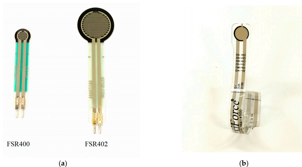
Figure 3. An example of the elementwise polymer thick film sensors (a) FSR sensors; (b) Flexiforce ® sensor.
