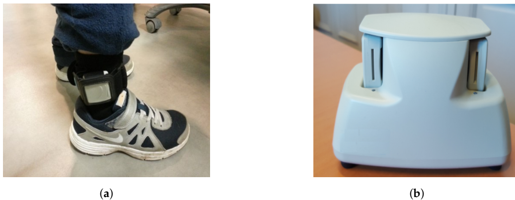
Figure 2. (a) WATA (Wearable Ankle Trajectory Analyzer) device worn at the ankle. (b) WATA devices connected to their case.
