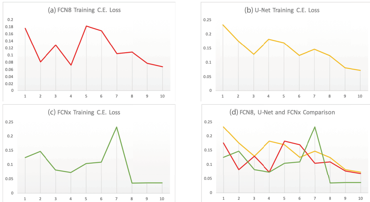
Figure 13. Comparison of FCN8 (a), U-Net (b), and FCNx (c) architectures training C.E. Loss over 10 training cycles (d).
