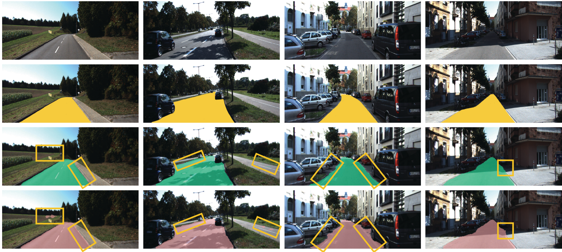
Figure 14. Results of semantic segmentation of the road. First row: some examples of road scenes in various situations. From left to right: Highway clear weather no traffic, highway shadow mix with traffic, urban dim with cars parked, and urban shadow mix with cars parked. Second row: the corresponding road ground truth annotations in yellow overlaid over the original image. Third row: road segmentation by our model FCNx. Row four: road segmentation by UC Berkeley FCN8.
