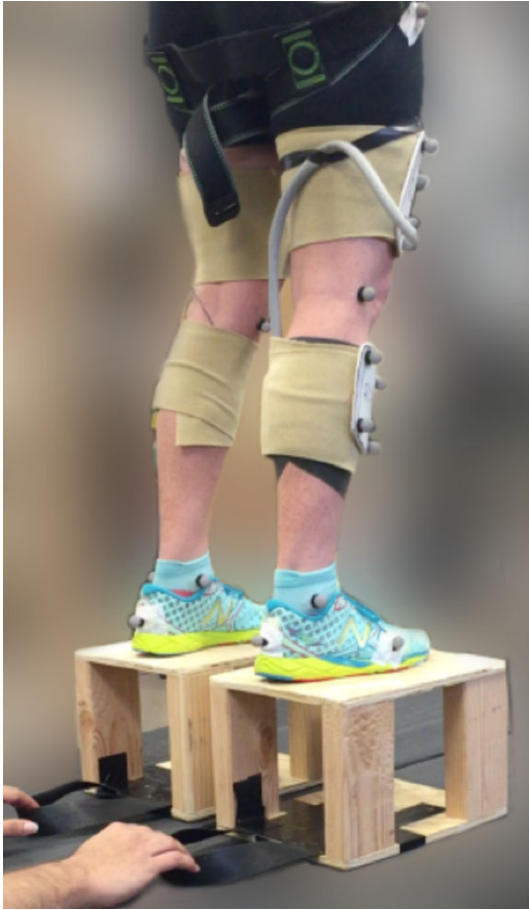
Figure 1. Experimental set-up for perturbation trials. Individuals hopped continuously at their preferred frequency ( 2.4 \pm 0.02 Hz) until an unexpected perturbation was elicited via manual removal of the custom-built platforms (20 cm height shown). Lower-limb kinematics were measured using motion capture and ground reaction forces were measured using a stationary split-belt treadmill. (Online version in colour.)
