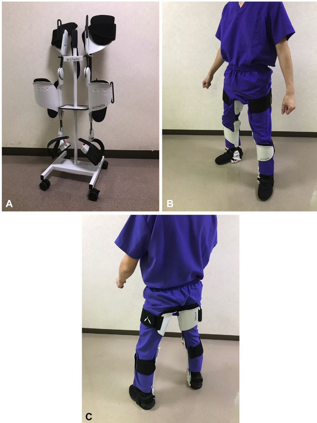
Figure 1. A, The Archelis wearable chair. B, Endoscopist wearing the Archelis (front view). C, Endoscopist wearing the Archelis (back view).
