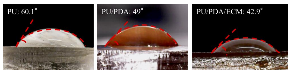
Figure 2. The water contact angle of PU, PU/PDA, and PU/PDA/ECM specimens.
