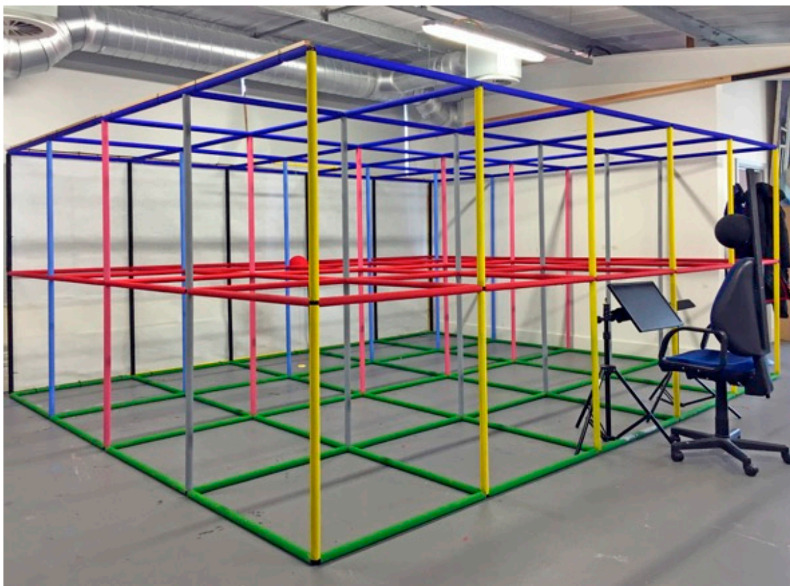
Figure 4. Experimental setup, showing the 3D grid room layout, the chair from which the scene was viewed, the location of the computer monitor, and the fixation sphere.
