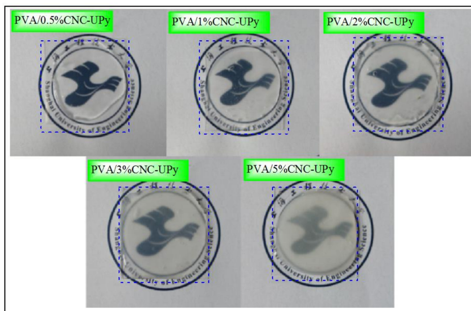
Figure 5. Photos of different PVA composite membranes.
