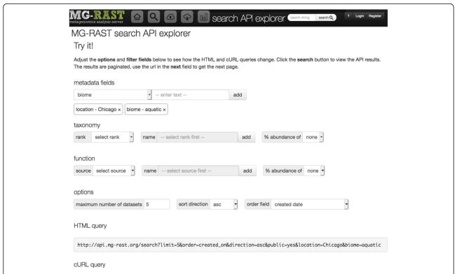
**Fig. 3** Using the API explorer to construct a query for aquatic datasets from Chicago. This query was built by selecting "location" from a drop-down menu, entering the value "Chicago," and selecting "biome" from the same menu and entering the term "aquatic." All the valid API options are presented as editable fields; the API's response to the query is shown in the gray box at the bottom of the page labeled "result from API."
