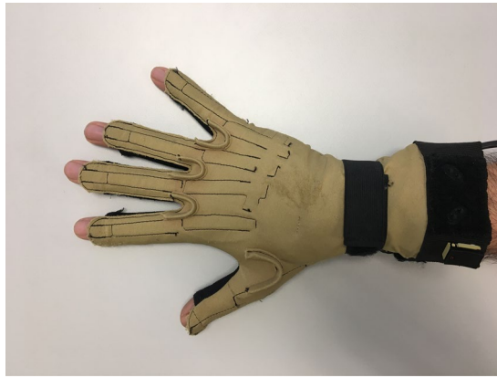
Fig. 1 Cyberglove I device and the strap used for the wrist sensors.
