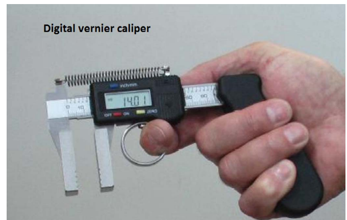
Fig. 3. Vernier calliper used for measuring the skin thickness before and after injecting bovine tuberculin antigen.
