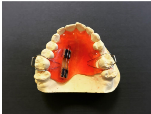
FIGURE 1 Intraoral appliance fitted with two enamel samples
