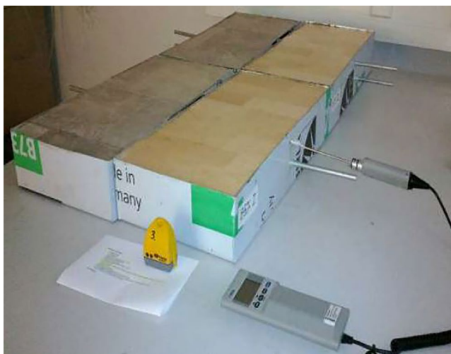
FIGURE 2 Measurement of the surface RH of one of the coated concrete slab
