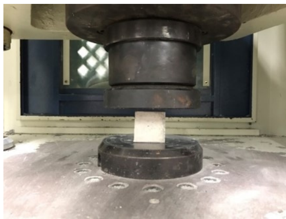
Figure 3. The illustration photo of compression test for cubic specimen.
