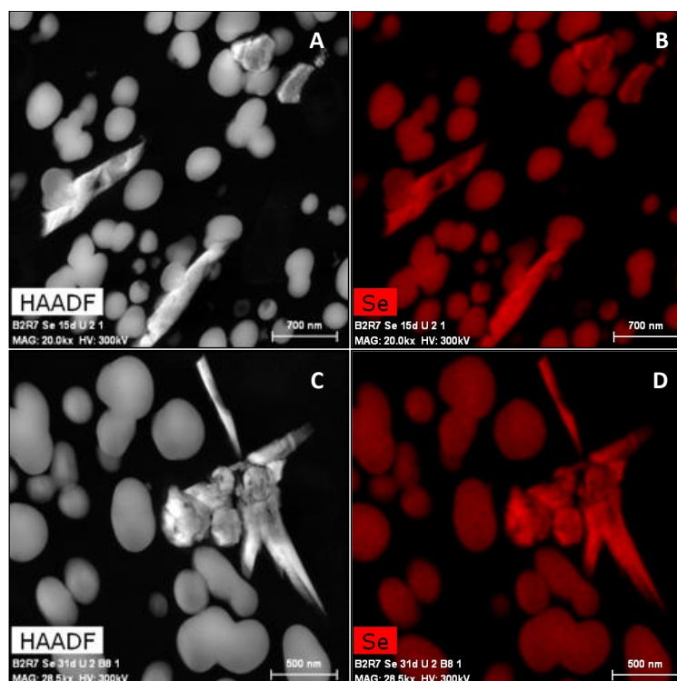
Figure 9. HAADF-STEM micrographs of Se nanostructures aerobically produced by S. bentonitica in the presence of 2 mM Se IV for 15 days (A–D). Corresponding elemental maps showing the Se composition of the nanostructures. Scale bars: 700 nm (A,B) and 500 nm (C,D).
