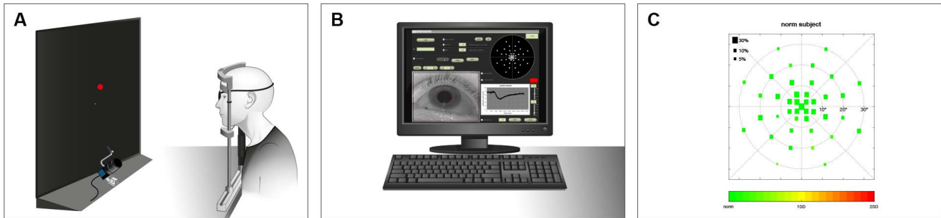
Figure 1. Pupil campimetry setup. Stimulus presentation on an OLED monitor (A). Examiner's monitor with stimulation details and pupil tracking (B). Result from a normal subject; cone protocol (C). The size of the squares represents the amplitude of pupil constriction after the respective local light stimulation. Color scale indicates deviation from mean of the group from green to red.
