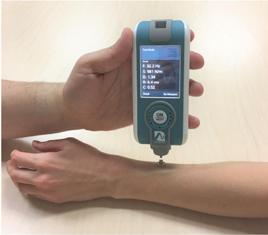
**Figure 1.** Myoton, a noninvasive handheld device, modified to isolate cutaneous tissue.
