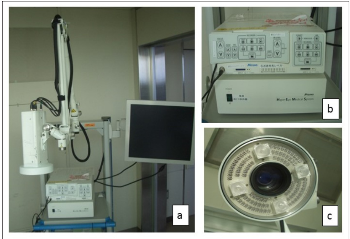
Fig. 1. Appearance of the HyperEye Medical System. a Overview of the HyperEye Medical System (Mizuho co.); b System for near-infrared fluorescent imaging; c Camera head used for fluorescent imaging.
