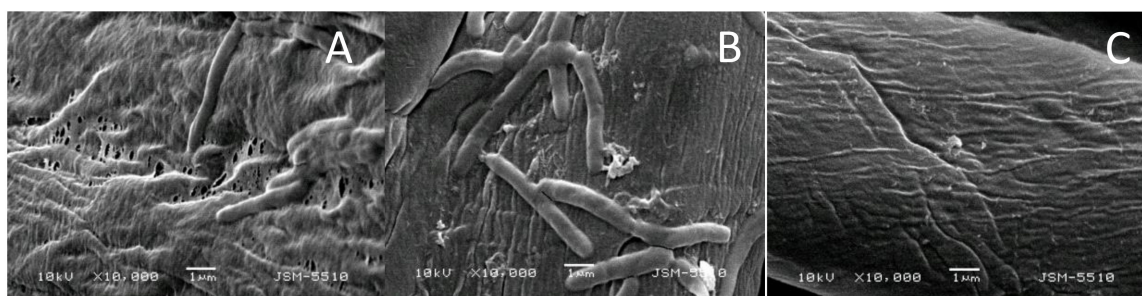
Figure 7. Scanning electron microscope (SEM) micrographs of cotton fabrics tested against B. cereus : cotton fabric before treatments (A), cotton fabric treated with BT (B), and cotton fabric treated with [Zn(BT)(NO_3)_2] (C).
