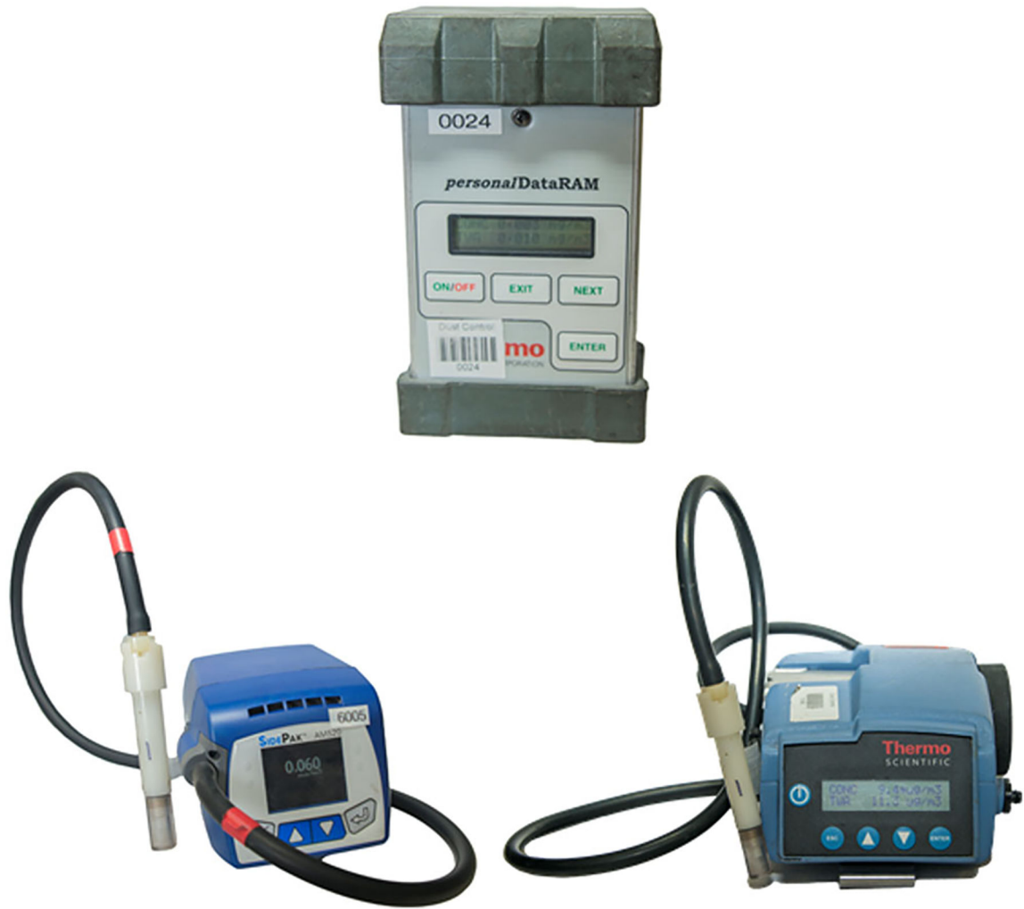
Fig. 1. Instruments tested—pDR-1000 (top), AM520 (lower left), and pDR-1500 (lower right)
