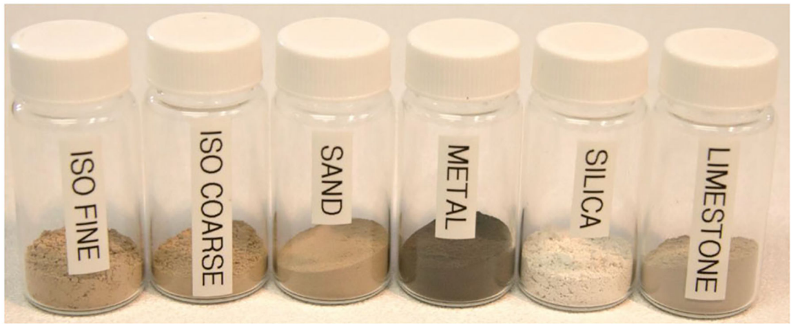
Fig. 2. Dust types used for the study, including ISO fine and coarse, sand, metal, high purity silica, and limestone
