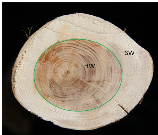
Figure 1. The heartwood and sapwood in T. chinensis (Pilger) Rehd. (HW: heartwood, SW: sapwood).
