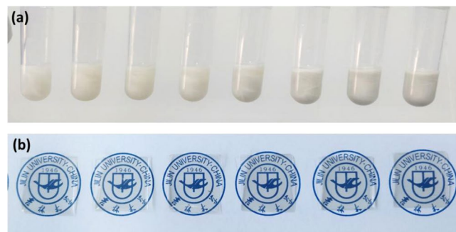
Figure 10. (a) Photographs of different concentrations of AgNWs (from left to right: 0.1, 0.2, 0.3, 0.4, 0.5, 1.0, 1.5, 2.0 mg/mL). (b) The Photographs of SLG-AgNWs composite films with different concentrations of AgNWs (from left to right: 0.1, 0.3, 0.5, 1.0, 1.5, 2.0 mg/mL), even at high concentrations (2.0 mg/mL).
