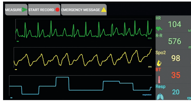
FIGURE 7: Interface display of monitoring parameters (application display).
