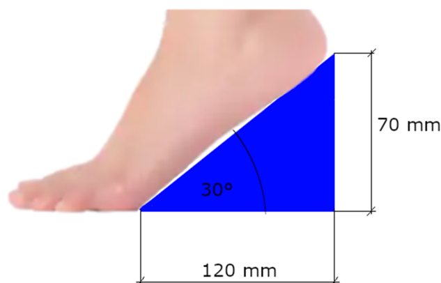
Figure 3. Schematic view of the wedge used as the heel with dimensions. The maximum height of the wedge was slightly larger than the heel effect it had on the foot.
