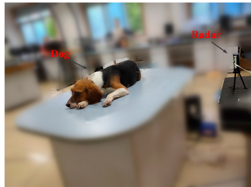
Figure 9. Setup for dog vital signs detection.
