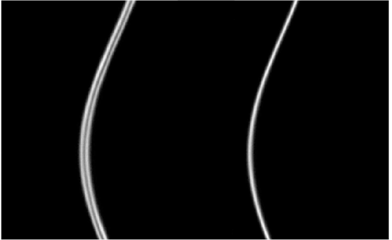
Figure 10. Sinogram of a point source before (left) and after (right) aligning the heads
