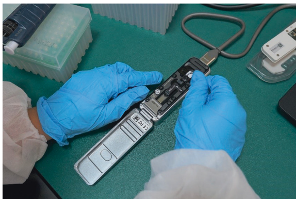
Fig. 1 The portable sequencer, MinION, is being handled prior to sequencing
