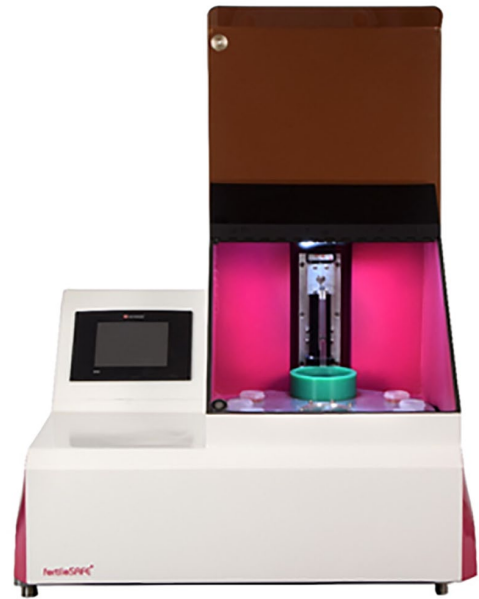
Figure 1. Schematic representation of the “Sarah” (FertileSafe Ltd, Israel) device for automation of the freezing process.
