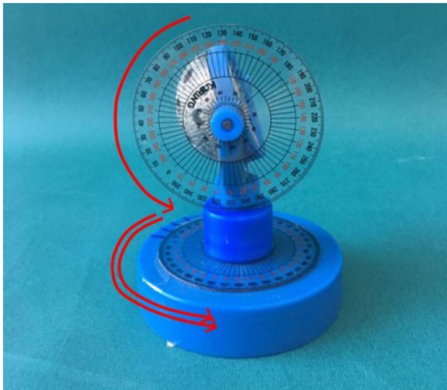
Fig. 1 Custom-made bi-planar anteversion measurement device allowing inclination and anteversion of the mounted cup with protractors in two axes. The solid arrow indicates the change in anteversion, while the hollow arrow indicates the change in inclination
