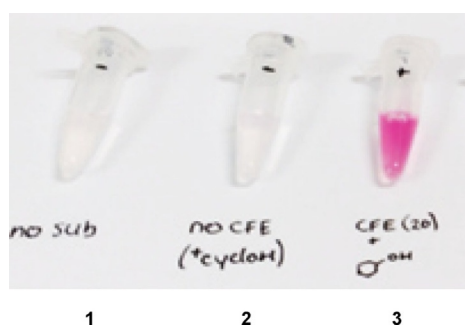
Figure 1. With an HRP-coupled assay, the alcohol oxidation activity of the NOX-A fusion can be detected without any addition of NADP + (3). The reaction mixture included buffer (50 mM Tris-HCl pH 7.5), HRP (0.8 U), AAP (0.1 mM) and DCHBS (1 mM), cell-free extract containing NOX-A (10% v/v) and 30 mM cyclohexanol. Controls: 1) no substrate and 2) no cell-free extract.
