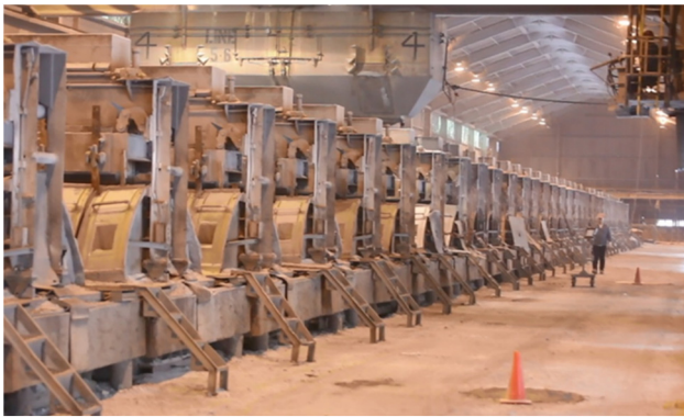
FIGURE 1 Aluminum smelter pot room showing a series of pots [Color figure can be viewed at wileyonlinelibrary.com ]
