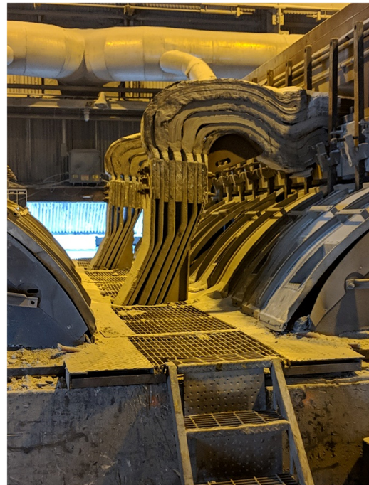
FIGURE 2 “Catwalk” between two sequential pots showing in-place covers over electrolytic bath [Color figure can be viewed at wileyonlinelibrary.com ]
