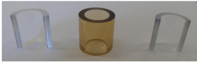
Figure 6: “As manufactured” KG-33 glass (left), KG-33 glass irradiated to 6 kGy (center), KG-33 glass irradiated to 6kGy and annealed as described in the text.
