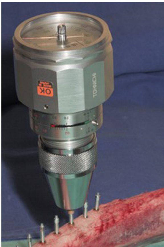
Fig. 1 Insertion torque and unscrewing device. Determination of insertion torque of individually hand-tightened smartpegs in test group by recording the removal torque required when unscrewing the device (BTG36N Analog Torque Meter, Tohnichi Manufacturing Co. Ltd., Tokyo, Japan)
