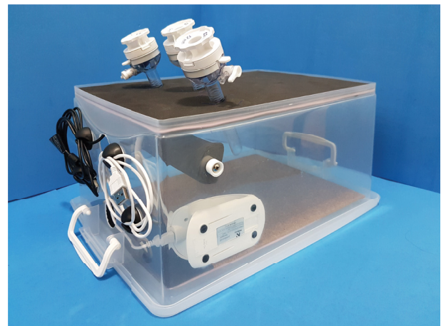
Figure 4 - Simulator final aspect: camera attached to the camera holder with cable tie. Flexible table lamp passed behind the camera holder with the LEDs pointing toward the center of the simulator.
