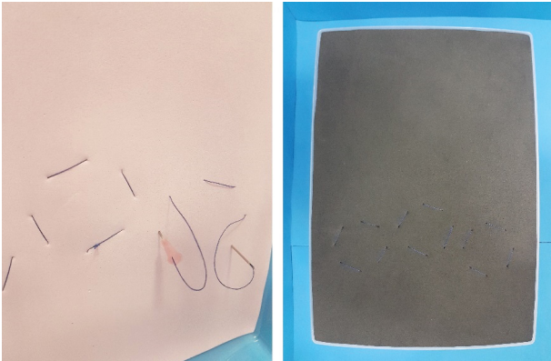
Figure 3 - Layers of EVA fixed with 2-0 cotton threads, by a 40.0 x 1.2 mm (18 G x 1 1/2") needle. Fixation through the 3 mm holes made around of the 32 mm holes at the bottom of the simulator.
