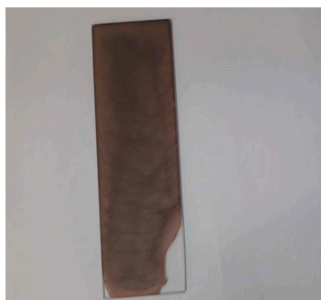
Figure 6. Photograph for deposited silver nanoparticles. The intense brown colour confirms the formation of Ag nanoparticles (NPs).
