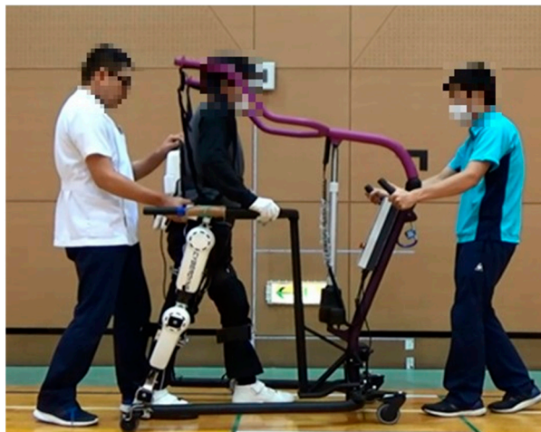
Figure 1. Walking exercise program using the bilateral (two leg version) Hybrid Assistive Limb® (HAL) robot.
