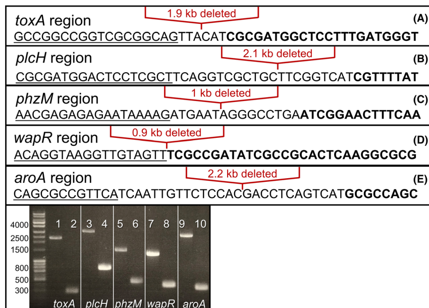
Fig. 1. Confirmation of deletion of five gene sequences in P. aeruginosa strain PGN5.
