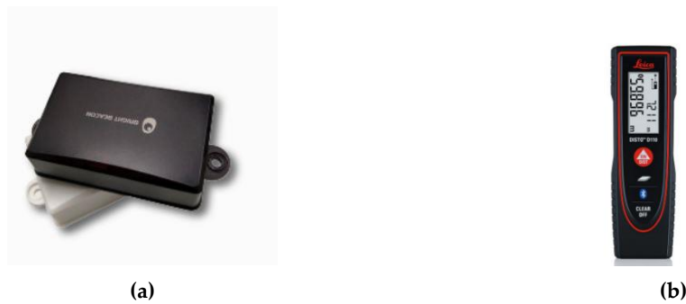
Figure 7. Experimental apparatus. (a) Max iBeacon from Bright iBeacon. (b) DISTO D110 laser distance meter from Leica Geosystems.
