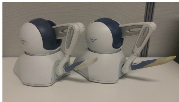
Figure 9. PHANTOM Omni haptic devices from SenAble Technologies. The company provided drivers and related software to utilize them.
