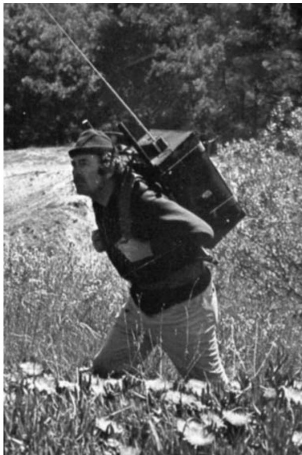
Figure 1. (A) Radiotransmitter in the form of an 85-pound backpack whose signal was carried a distance of one block.
